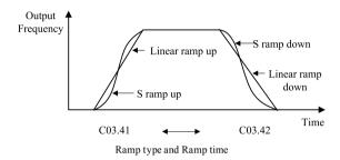
Attention: It is possible to switch acceleration and deceleration via digital input terminals, see parameterC05.1\* choice. The state of the digital input terminal is shown in binary code; If the drive detects the corresponding digital input terminals connected, then the bit is "I", on the contrary is "0". The corresponding relationship between state of the digital input terminalsbinary code and the selected ramp type are as follows:
