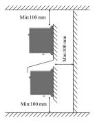
Fig. 3 Upper and Lower installation
