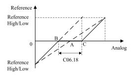
Description of Choice: Point A as shown in the figure is the analog value that corresponds to a setpoint that equals 0. It is calculated via analog low, high values and low, high references. UAB=UAC=C0618/2
