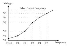
Fig. 6.1 V/F characteristic diagram
