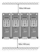
Fig.2 Side by side installation
